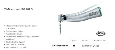
nano Series instruments are compatible with NSK motor line up (NLX nano, NLX plus, M40LED, NBX, NBX N, X205L, M205LG and SGL70M micromotors) and other motors with insert less than 23 mm.
