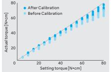
Minimizing the discrepancy between the set torque value and the actual output helps improve treatment outcomes.
